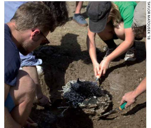
Students gently remove the dirt from the aluminum casting still in the ground.
