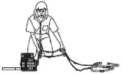
Use the plastic strap (attached to the bottom rung) to wrap and secure both layers of rungs. This will minimize the chance of the ladder becoming tangled when you remove it from the box in an emergency.
