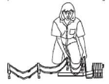
Stack a second layer of rungs 12 thru 22 on top of the bottom layer.
