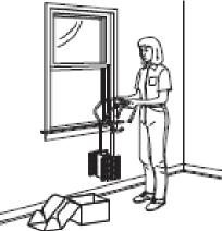
Place the sli hooks firmly over the windowsli and pull the release strap to deploy the ladder.
