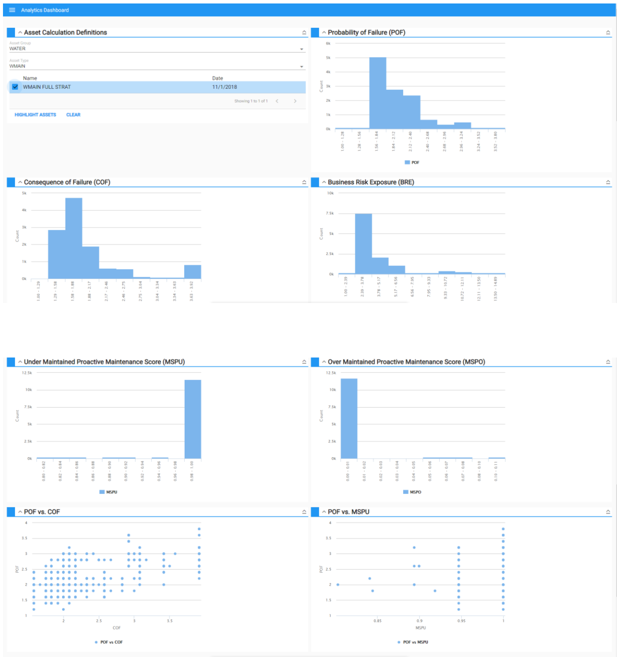
Figure 25 – Cityworks Analytics Dashboard presenting the water system business risk exposure level and KPIs to track asset management efforts.
