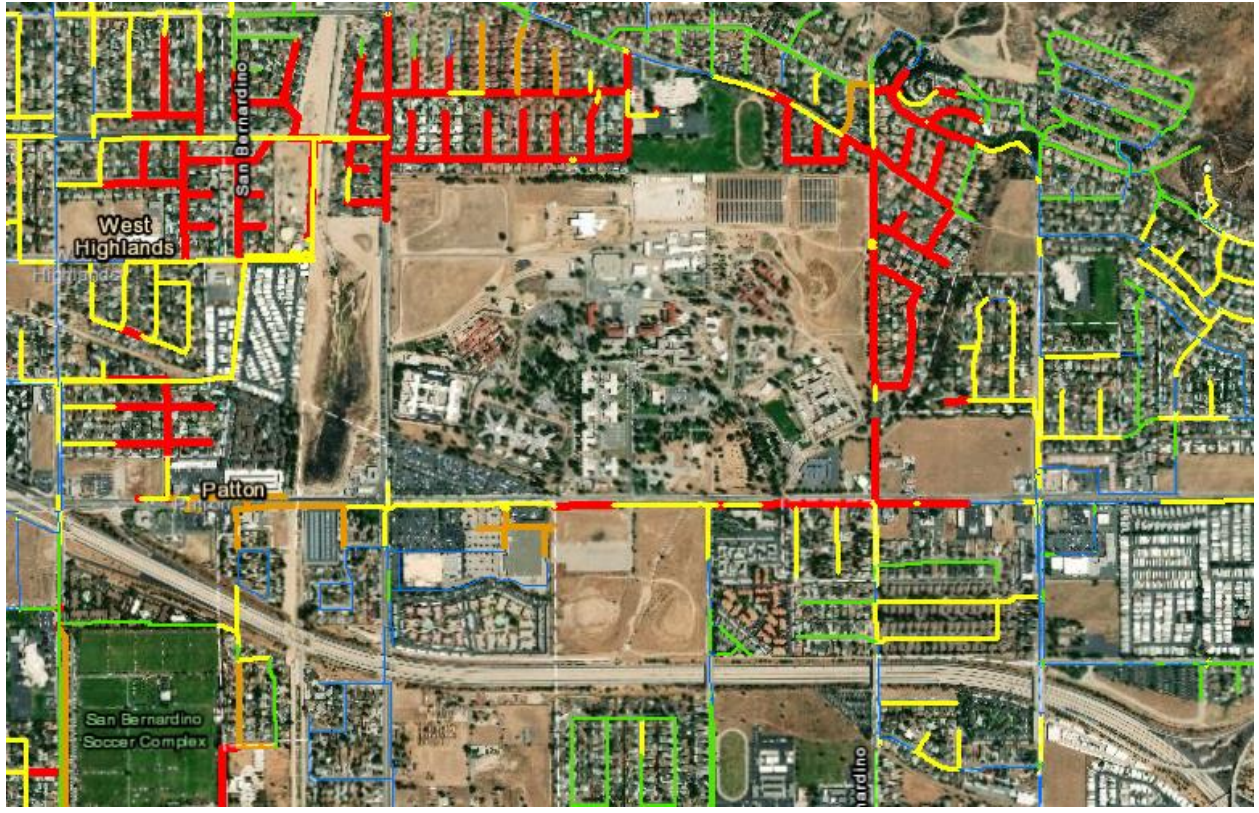
Figure 14 - Water mains symbolized based on consequence of failure due to number of meters impacted.
