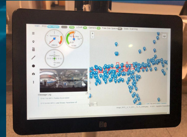
TIMMS interface showing scanned path and 360° image capture locations
